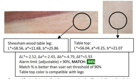
Sensegood Spectrophotometer for color management and quality control in wood products Determining color compatibility for wood products assembly
